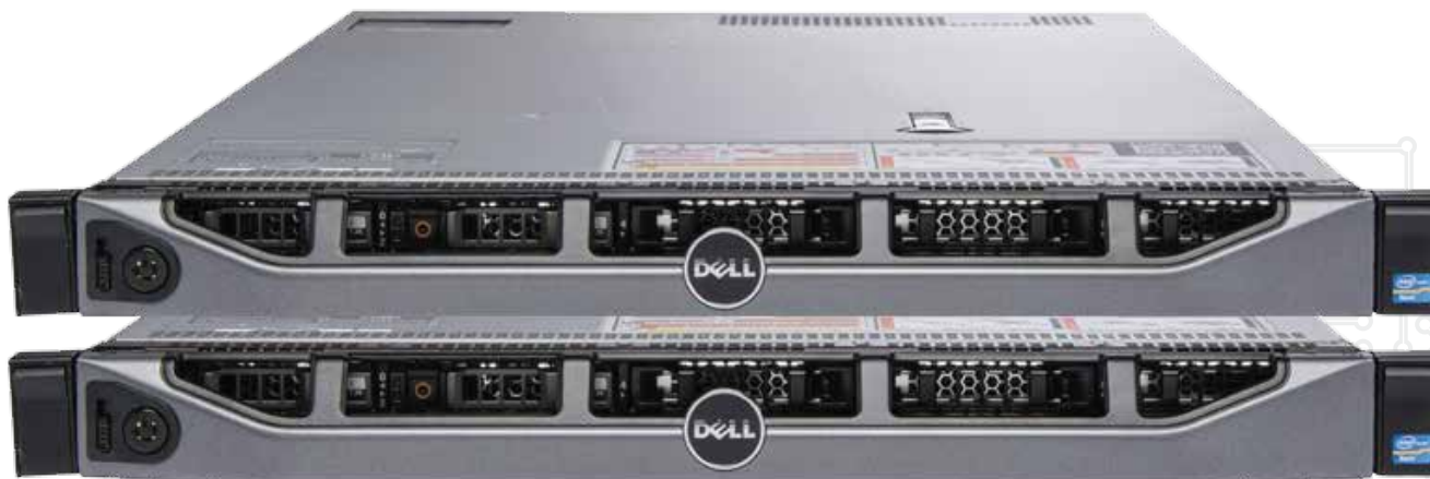
Owl Uses a Pair of Dell PowerEdge R620 Servers
